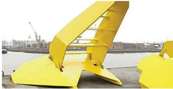
fig. 12/ two piece drag embedment anchor
