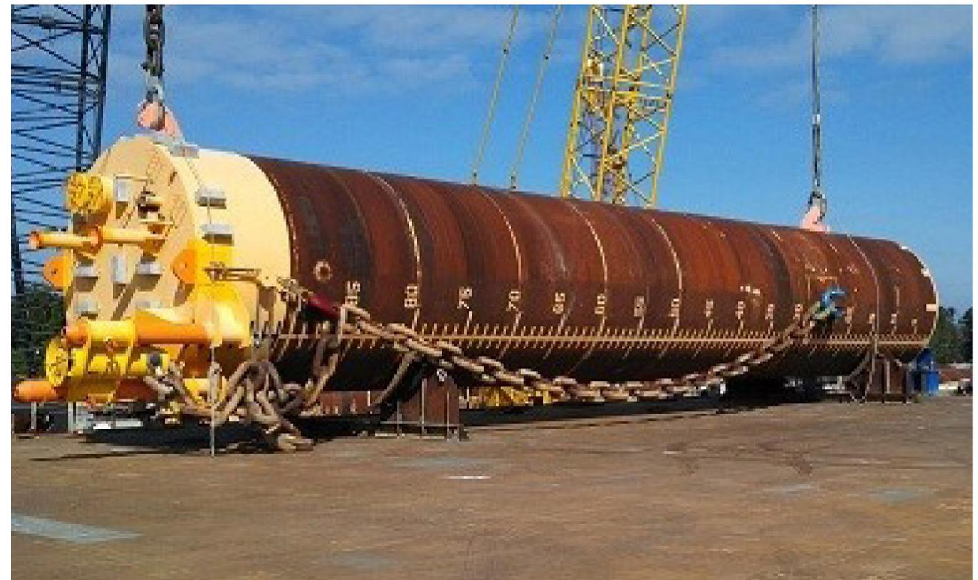
fig. 14/ suction pile anchor
