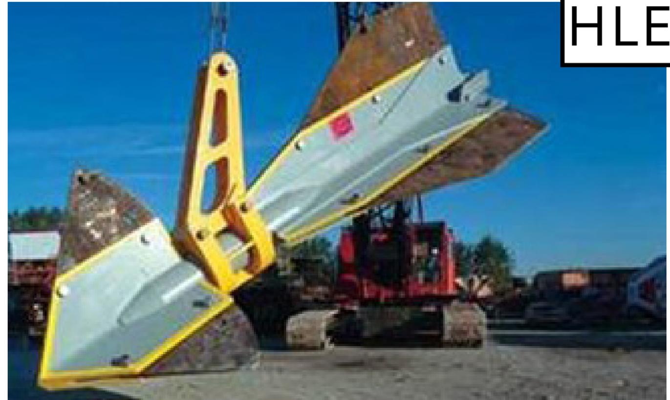
fig. 13/ drive pile anchor lifted by crane
