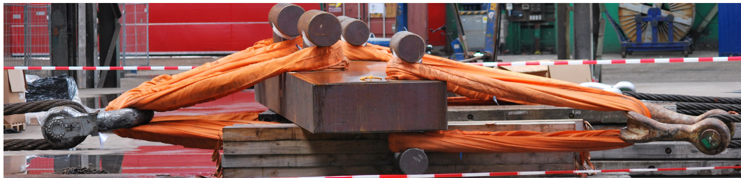
fig. 22/ lift being under test load
