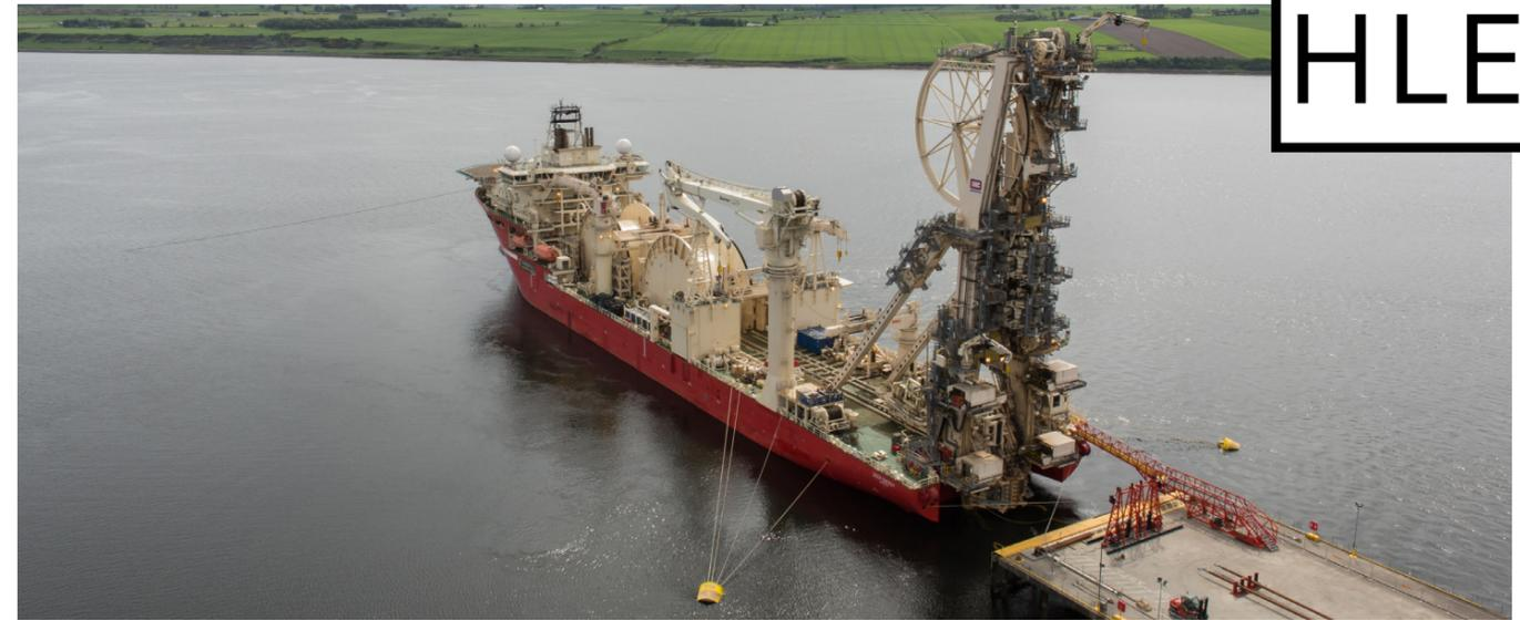
fig. 09/ pipelay vessel moored to bespoke mooring bouys
