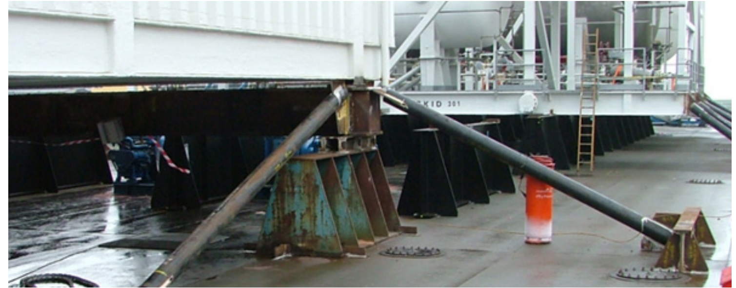
fig. 9/ typical detail for roll and pitch bracing common 'hard point' on the cargo
